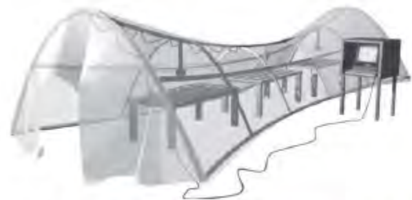
Fig. 23. Annual circulation greenhouse tunnel dryer [31].
